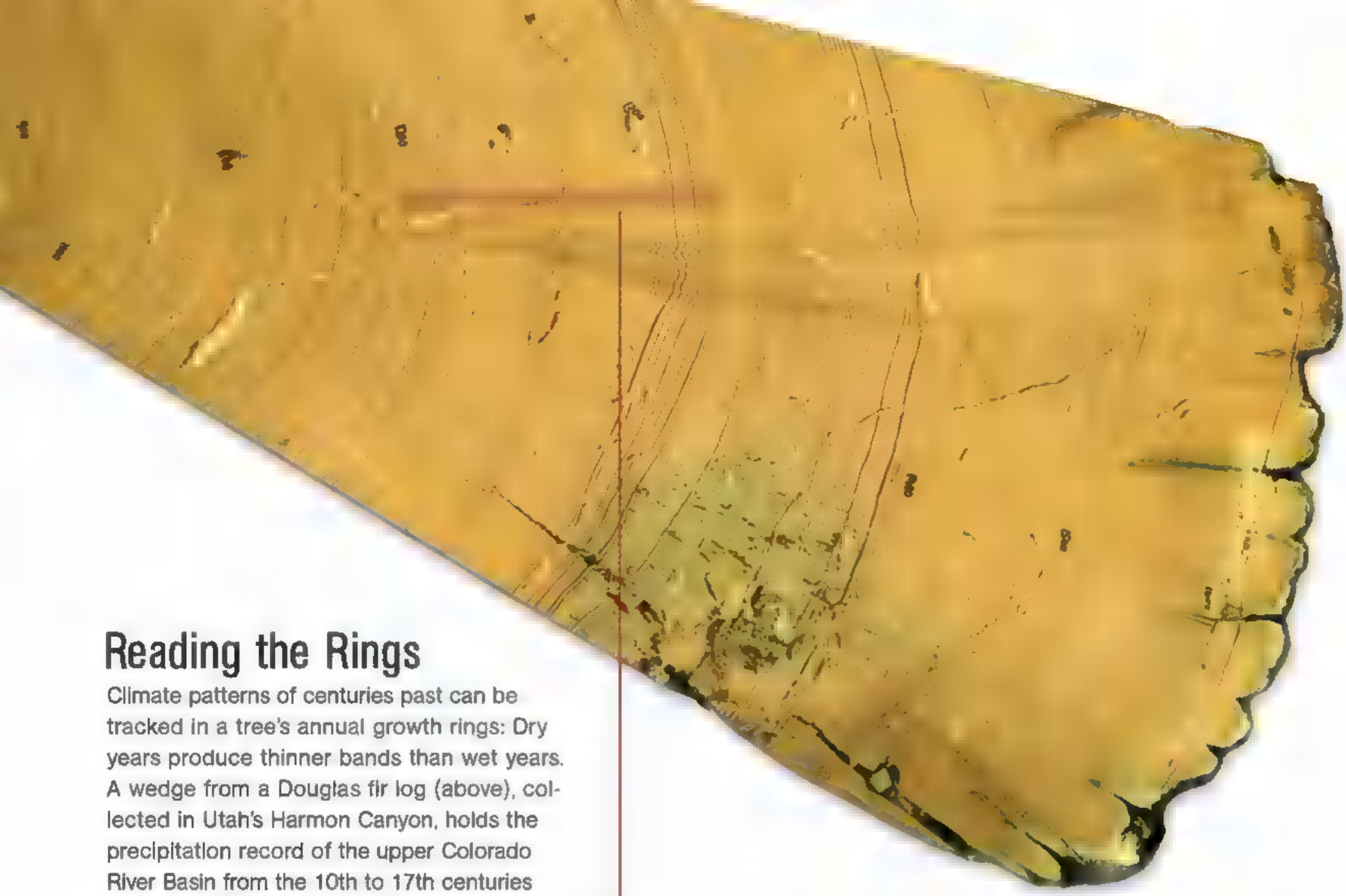
PHOTO: LABORATORY OF TREE-RING RESEARCH, UNIVERSITY OF ARIZONA. LENGTH OF WEDGE SHOWN IS 12 INCHES
